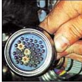
Figure 3.0: Hydraulic Fluid Damage
